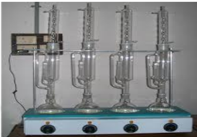
Figure 4. The experimental set-up of Micro-Kjeldahl Apparatus
