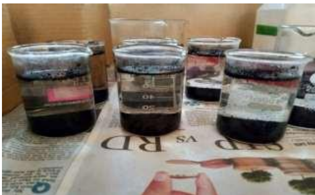
Figure 2. Water samples coagulation with rice husk ash
