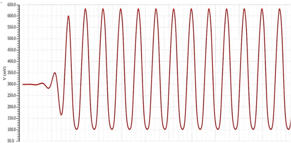
Figure 8. Output waveform of 3-stage ring HDCRO
