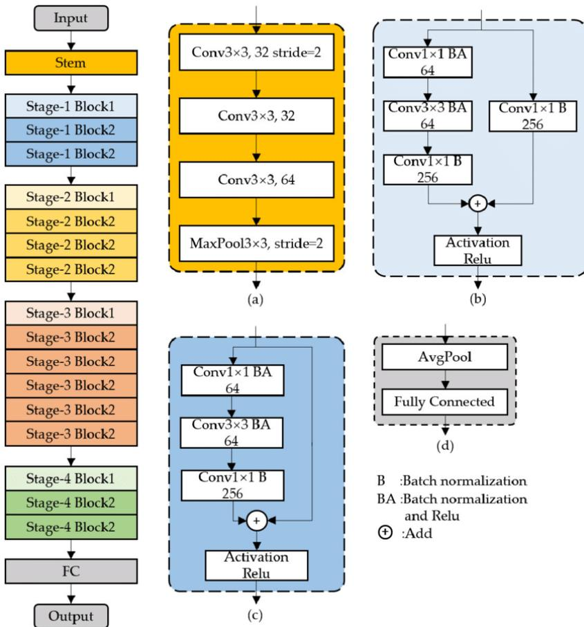
**Figure 4.** Architecture of the ResNet50
