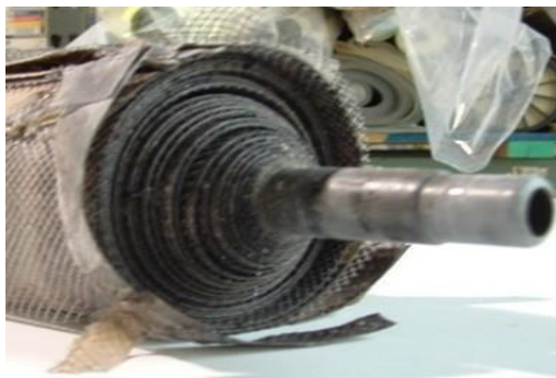
Figure 6. Large opening in the UF membrane of the UF element.
