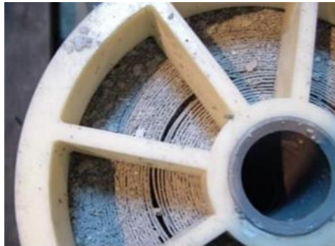
Figure 6. Large opening in the UF membrane of the UF element.
