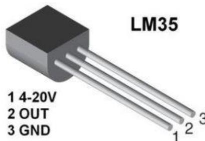
Figure 3. LM35 Temperature Sensor
