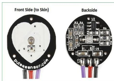
Figure 2. Pulse Sensor
