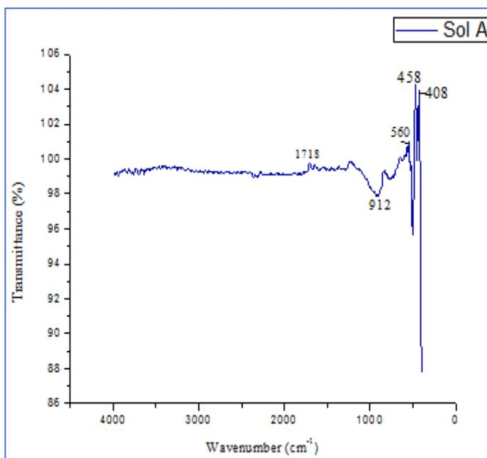
**Figure 5** FTIR spectrum of Sol A sample
