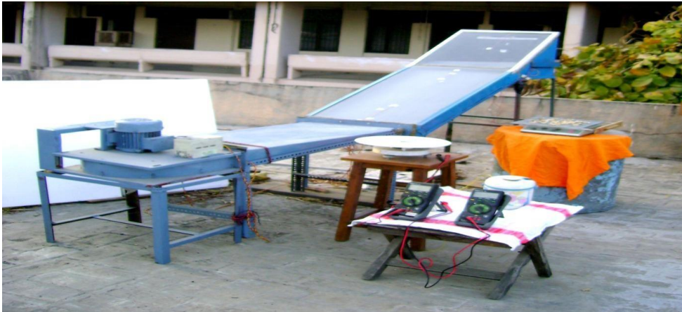
Figure 8. Experimental Set-Ups for Forced Convection Mixed Mode Solar Dryer in Real Climatic Condition.
